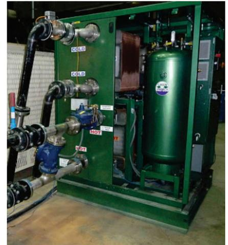
**ElectraTherm Green Machine ORC turbine**
