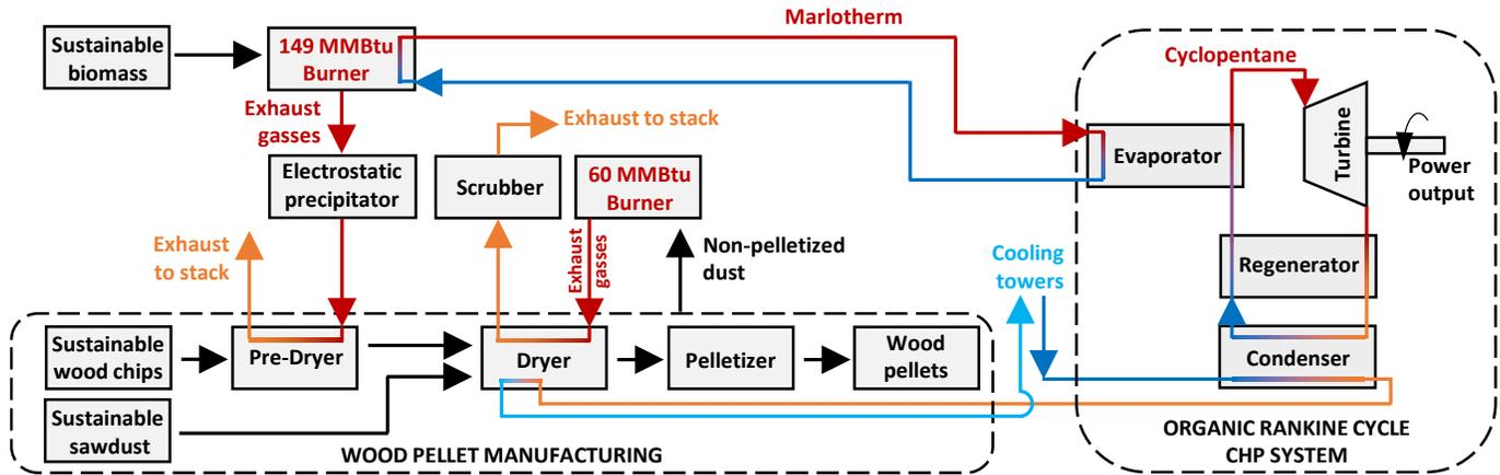
**Schematic of Maine Woods Pellet's pellet manufacturing and ORC CHP system**
