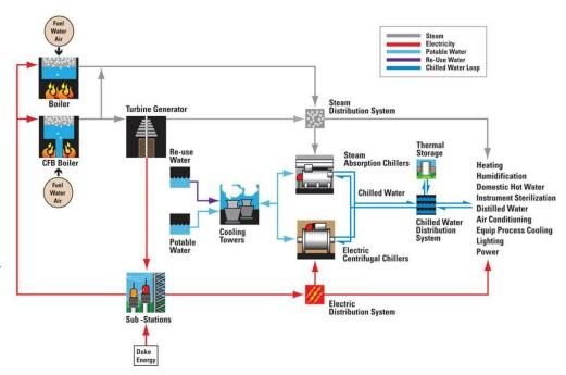
provide the greatest efficiency. The system controls the boilers and chillers remotely and runs an algorithm to choose the most efficient arrangement of equipment to have online.
